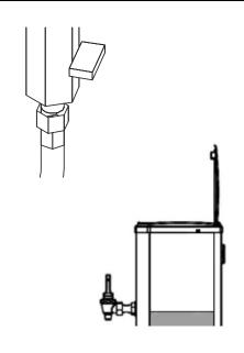
**1.2.** Connect to the Cold water supply using the hose provided. The most appropriate connection is to a tap that can be turned off.
